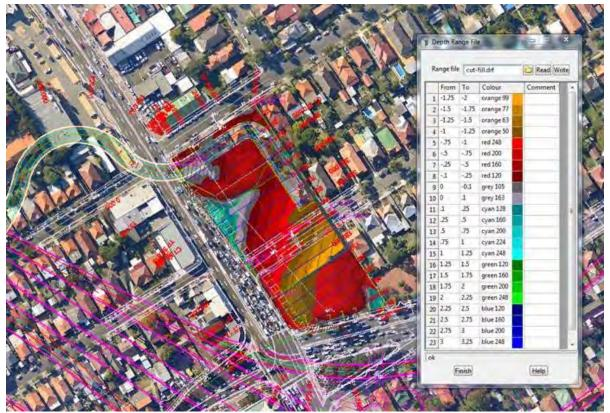
Figure 2: Proposed depth of excavation. Supplied by CSJ to Ramboll Environ
