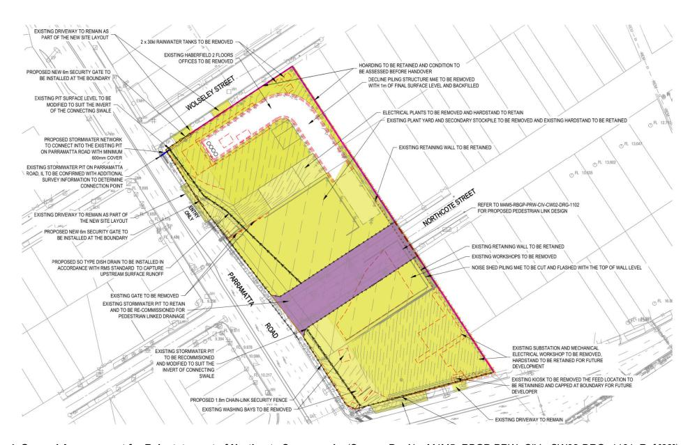
Figure 4 General Arrangement for Reinstatement of Northcote Compound (Source: Drg No: M4M5 -RBGP-PRW- CIV - CW02-DRG- 1101, Ref [63])
