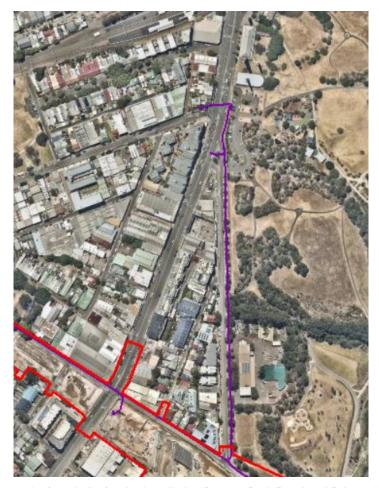
Figure 1: Location of ITS cabling works (purple line) to be installed at Barwon Park Road and Princes Highway. New M5 project boundary is shown in red.
