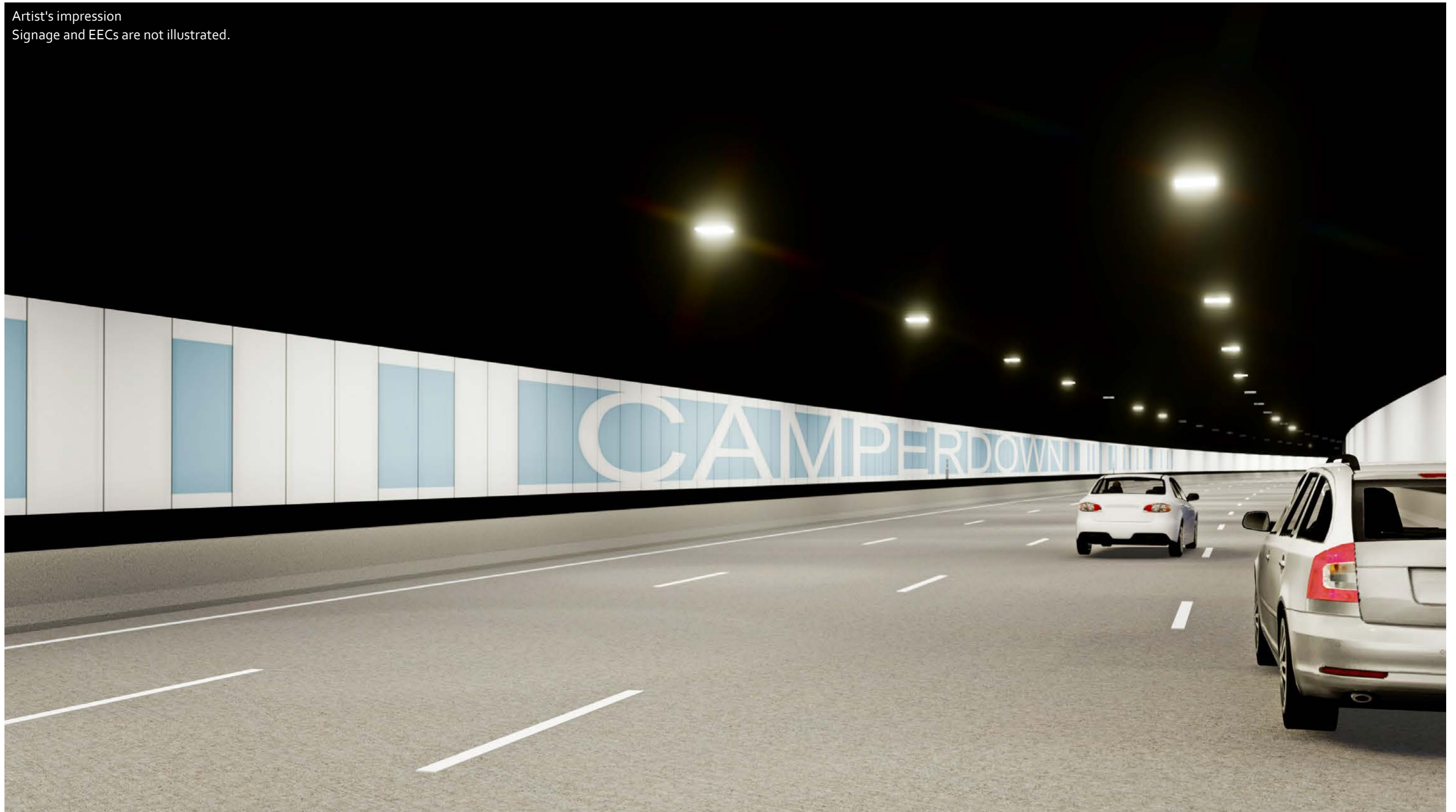
Figure 6-7: Tunnel location marker
