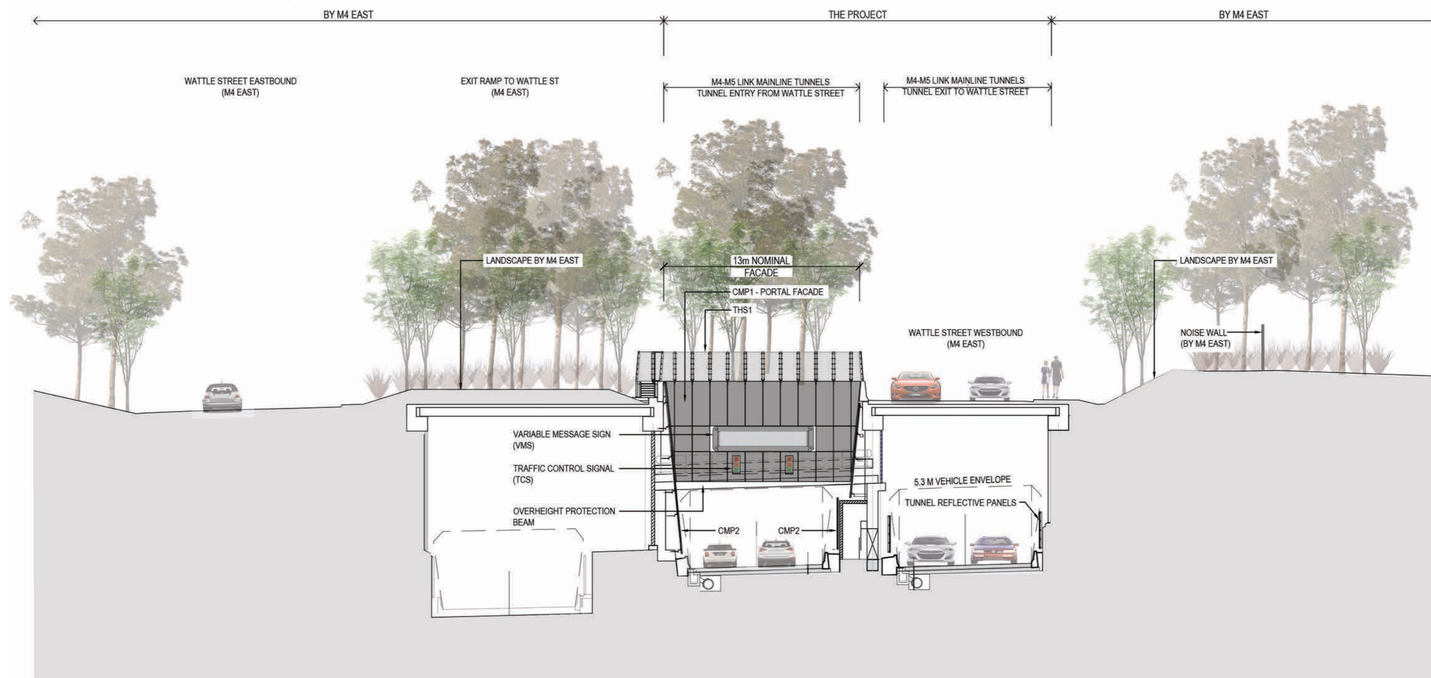
1 ELEVATION - ENTRY PORTAL FACADE SCALE 1:250
