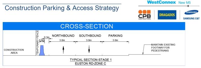
Figure 3: Stage 1 Construction Works in Euston Road
