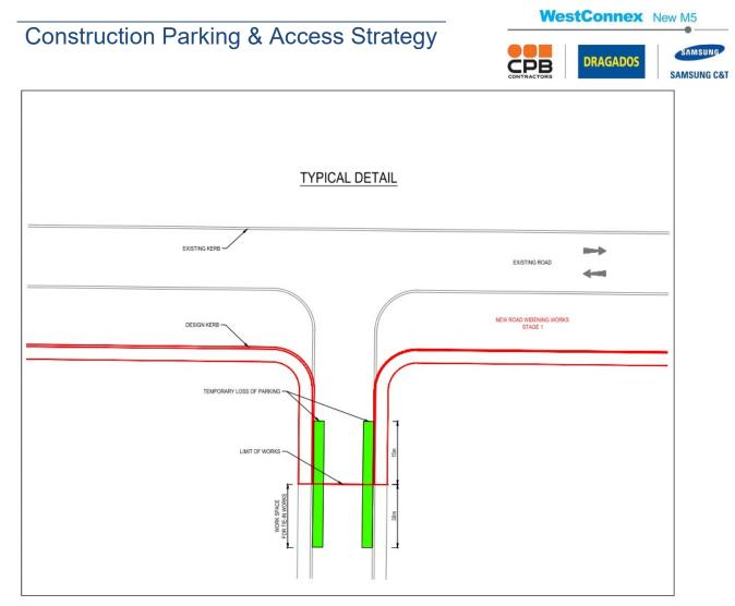
Figure 2: Typical details for side road and tie-in works
