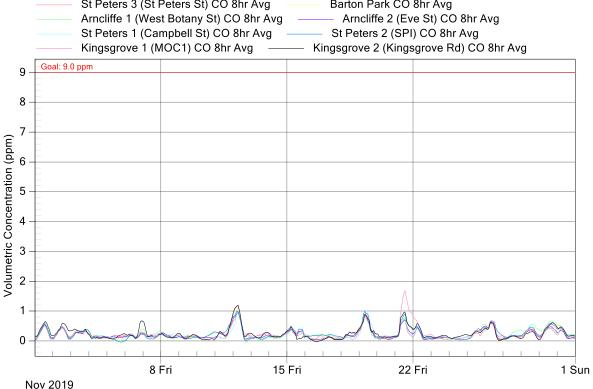
Figure 2: New M5 Project Air Monitoring Stations - CO 8 hours rolling graph for November 2019
