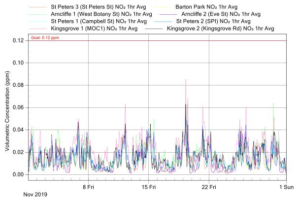
Figure 3: New M5 Project Air Monitoring Stations - NO<sub>2</sub> graph for November 2019
