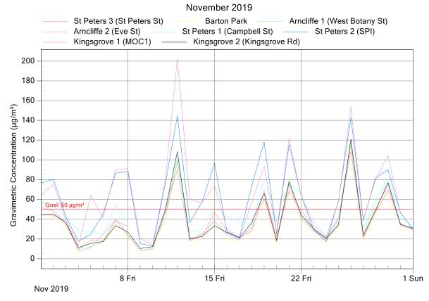
Figure 4: New M5 Project Air Monitoring Stations - PM<sub>10</sub> 24 Hour graph for November 2019
