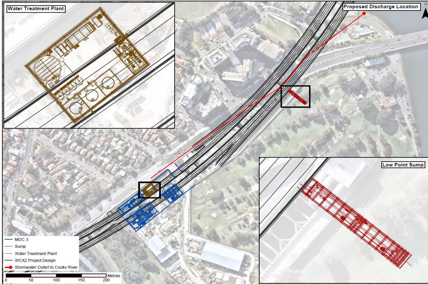
Figure 9: Operation water treatment plant, water tidal basin and discharge point
