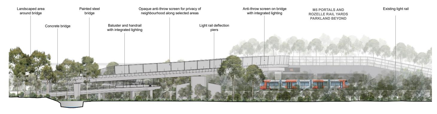
Figure 8-7: Section through Bridge to Brenan Street
