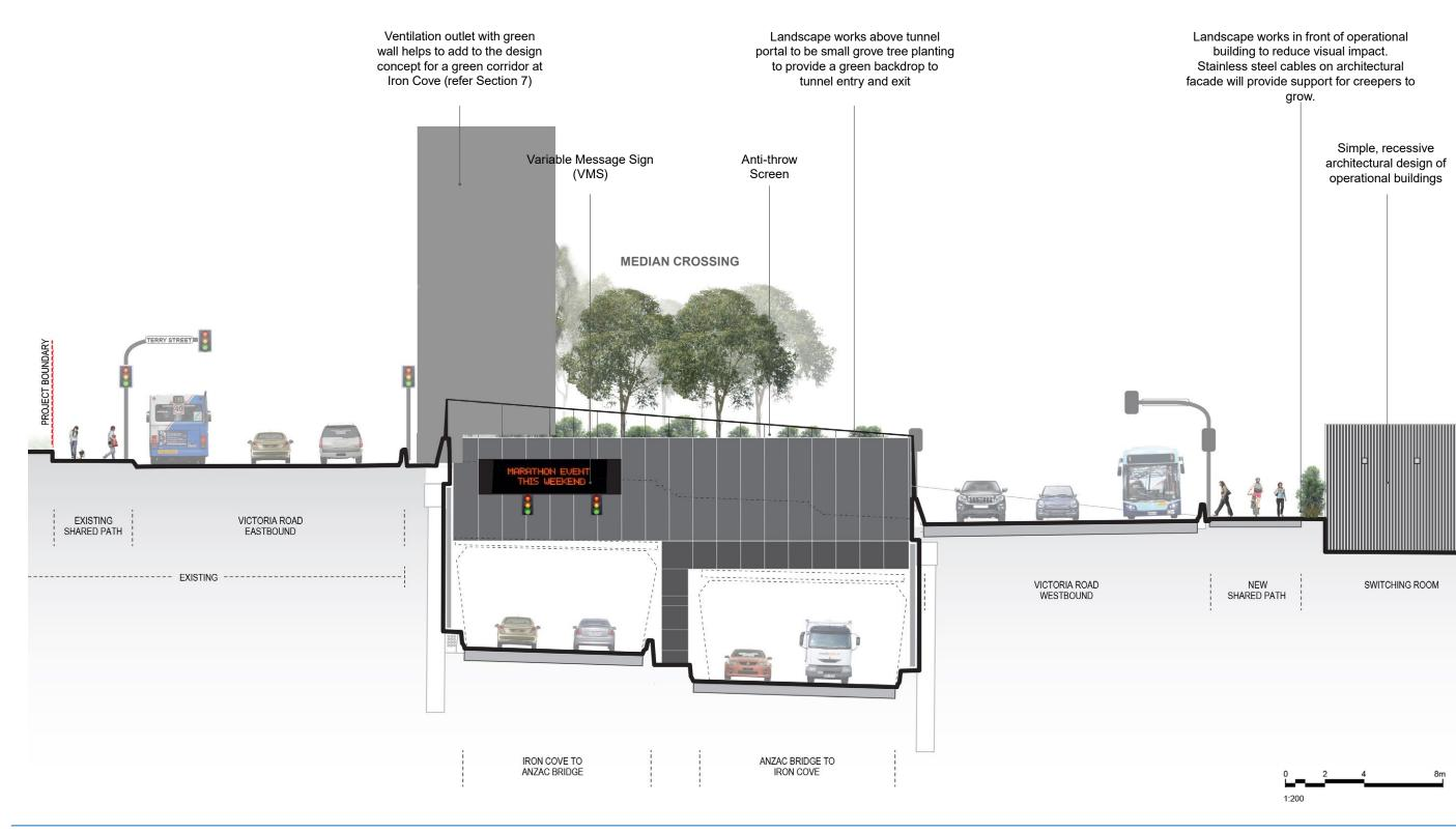
Figure 6-23: Iron Cove Link - Tunnel portal elevation
