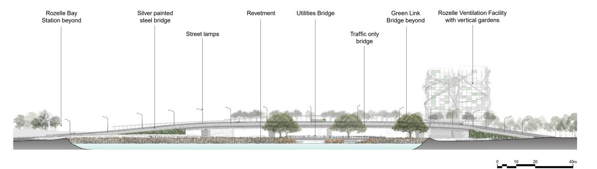
Figure 8-12: The Crescent Overpass: East sectional elevation
