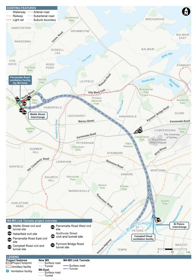
Figure 1-1 Key features of the M4-M8 Link
