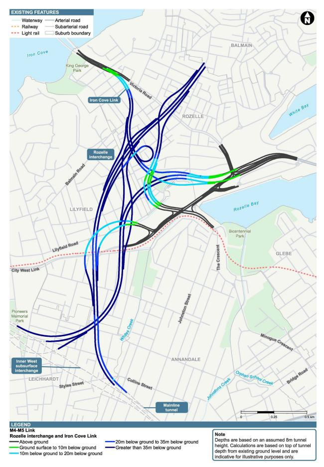
Figure 1-2 Overview of the Rozelle Interchange
