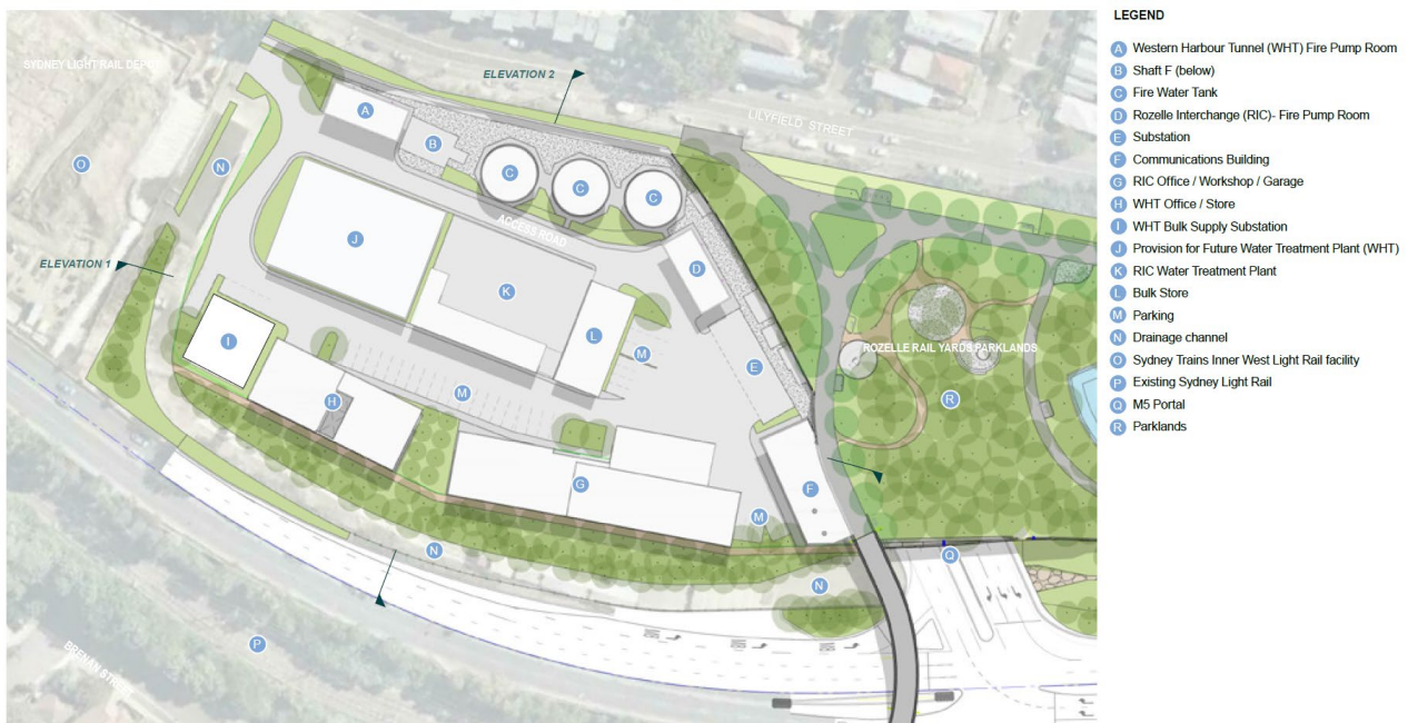
Figure 2-2 Motorway Operations Centre
