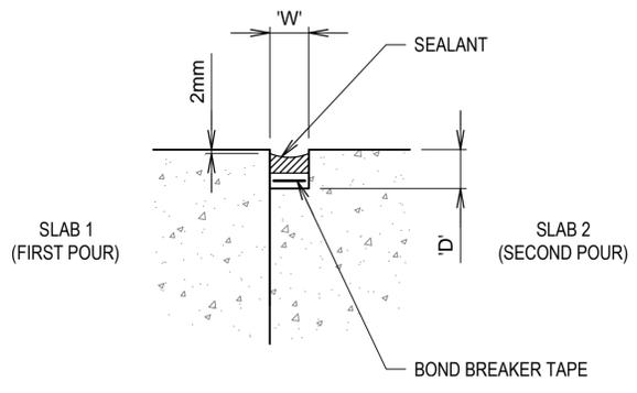
**MOVEMENT JOINT SEALANT DETAILS**
