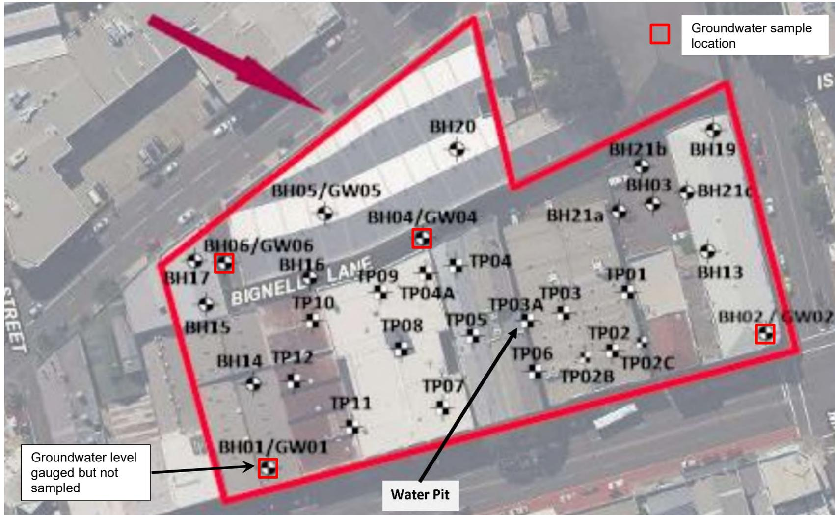
Figure 2-11 UST Sample Locations Used by Alliance 2019 DSI at PBR site
