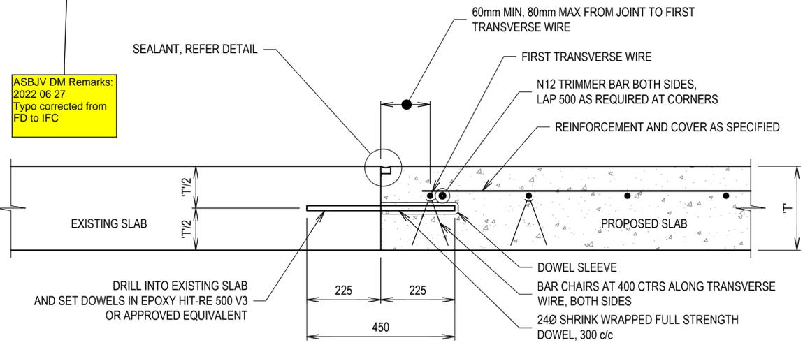
**CONCRETE REPAIR INTERFACE DETAIL**
