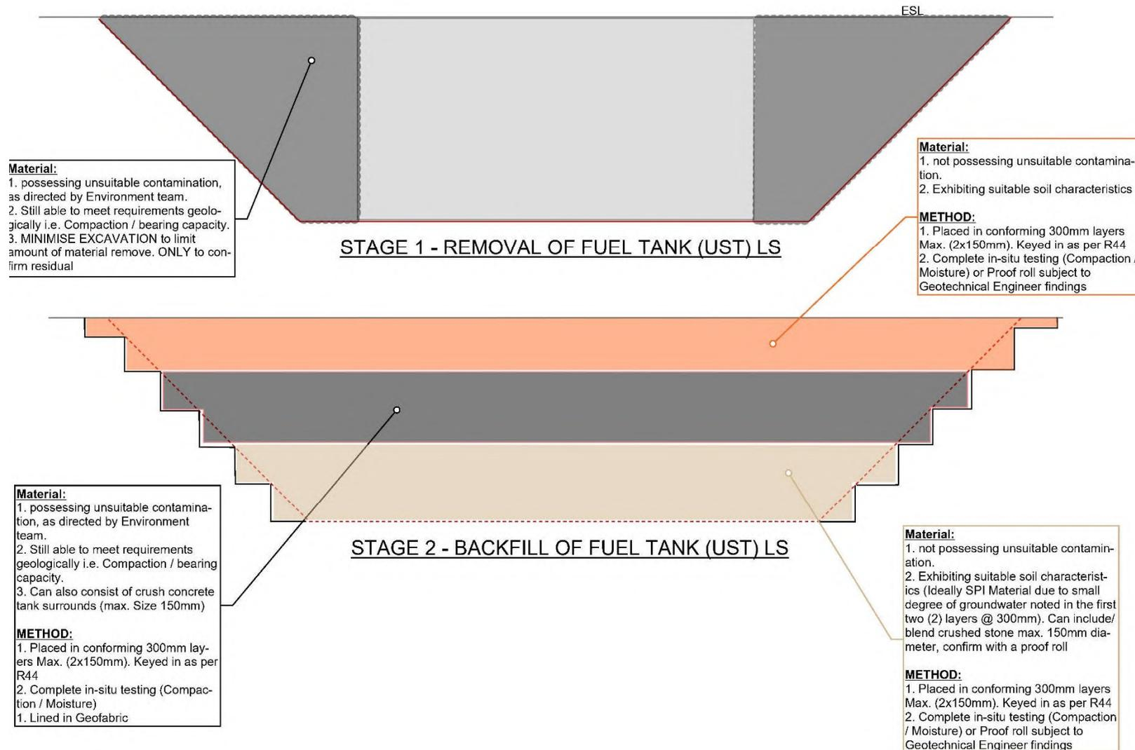
**Figure 3-4 ASBJV Methodology for Removing USTs & Excavation Backfilling (page 2 of 2)**
