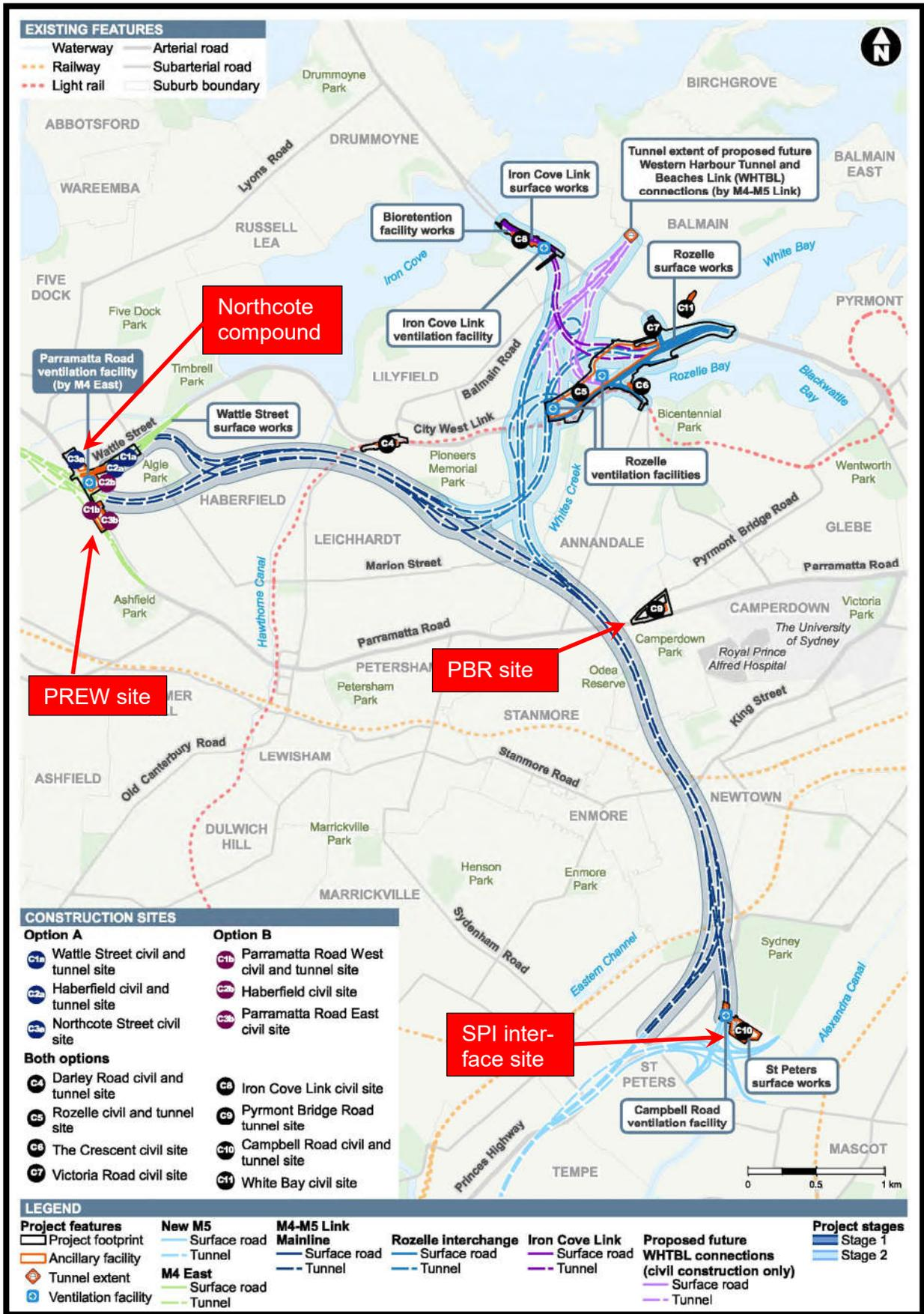
Figure 1 Overview of Project Footprint and Construction Ancillary Facilities (Source: Ref [50])
