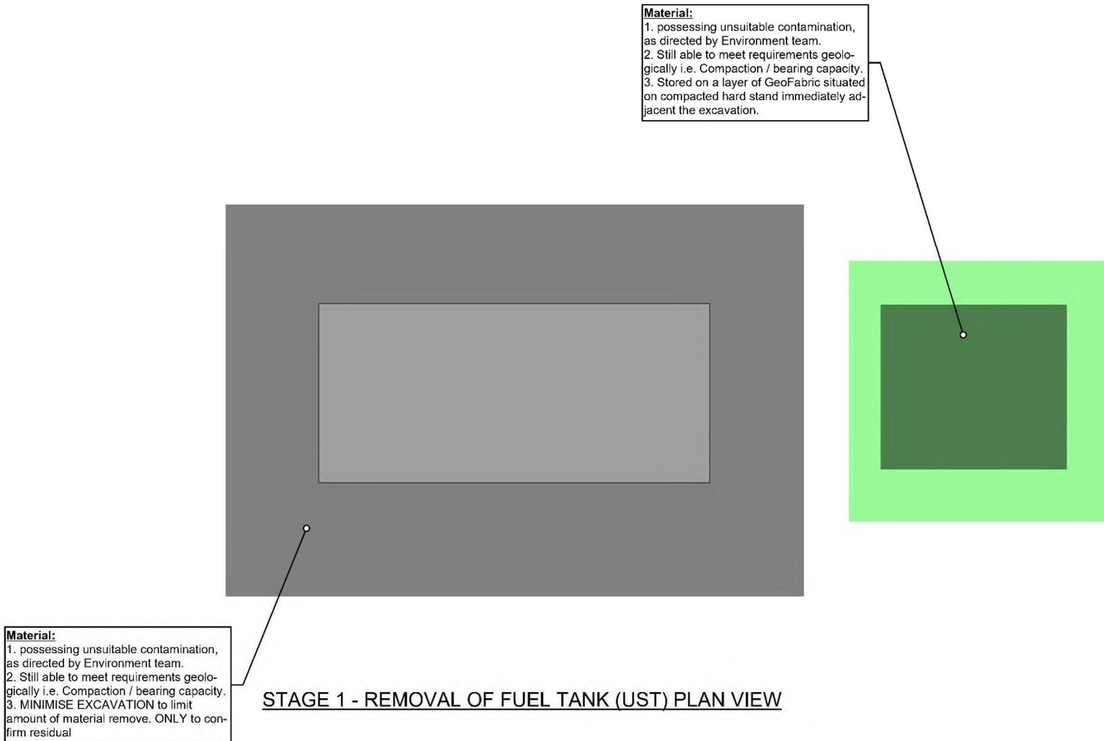
Figure 3-5 LSBJV Plans for Removal of Known USTs (page 1 of 3)
