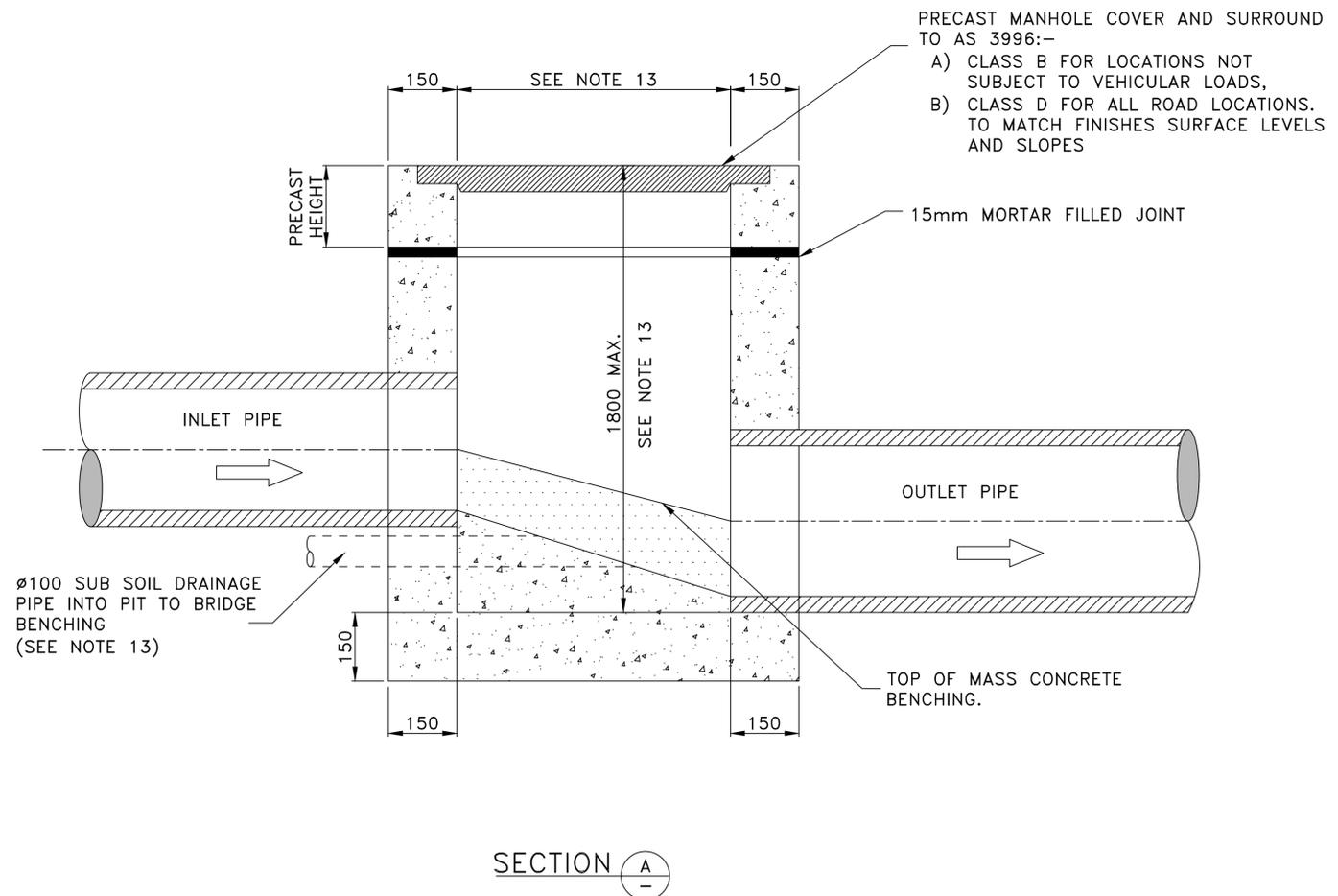
Ø100 SUB SOIL DRAINAGE PIPE INTO PIT TO BRIDGE BENCHING (SEE NOTE 13)
