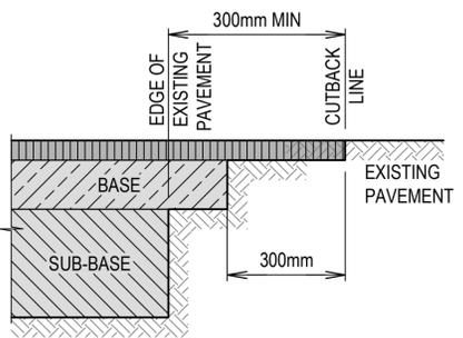
**TYPICAL EXISTING PAVEMENT CUT-BACK DETAIL**
