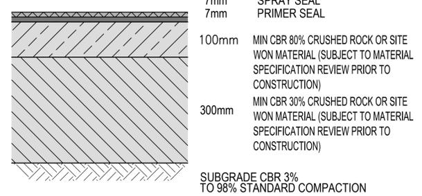
**FLEXIBLE PAVEMENT HARDSTAND**
