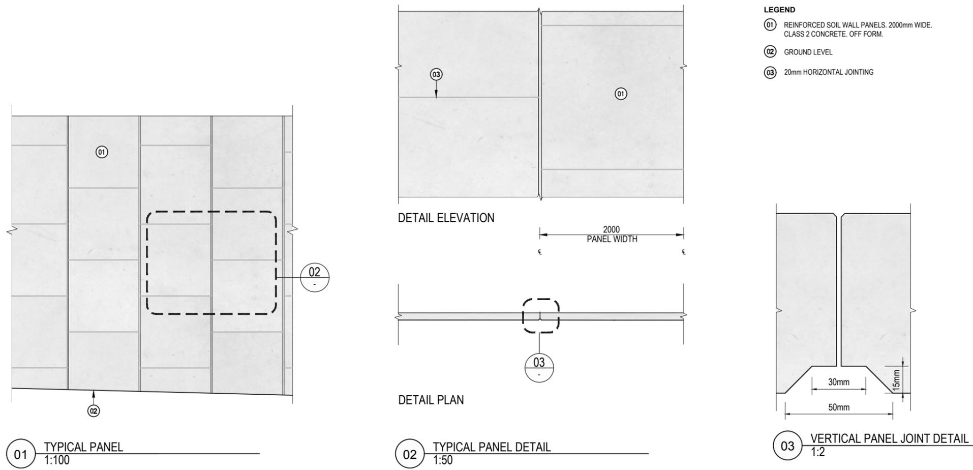
Figure 3-2 - Retaining wall typical details - Type 2B
