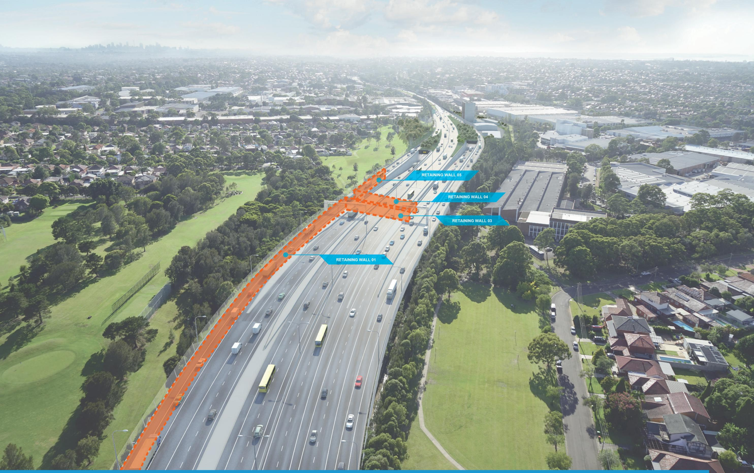
**AERIAL VIEW OF WESTERN INTERCHANGE AND PORTALS HIGHLIGHTING THE LOCATION OF RETAINING WALLS 01 AND 05 WHICH ARE LOCATED ON THE OUTER EDGE OF THE NEW M5 EASTBOUND BYPASS RAMP NEARSIDE SHOULDER, WITH 03 AND 04 UNDER THE BYPASS RAMP AT KINDILAN UNDERPASS.**
