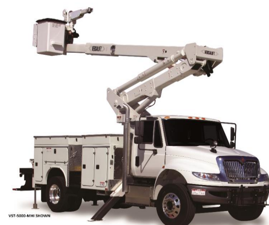
Image: a bucket truck used by technicians for overhead powerline work.
