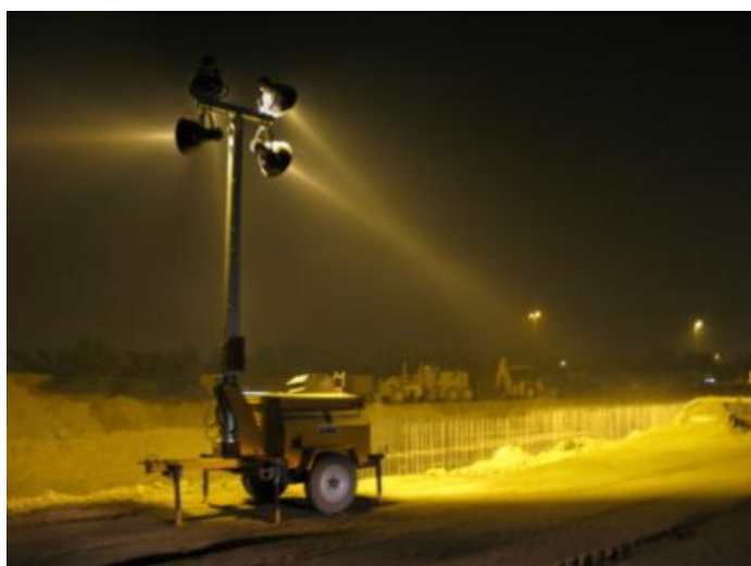
Image: Temporary lighting tower typically used during street lighting outages
