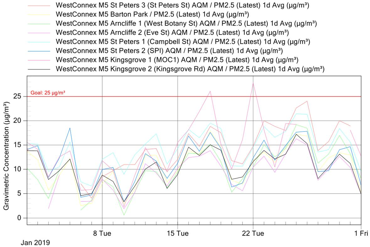
Figure 5: New M5 Project Air Monitoring Stations - PM<sub>2.5</sub> 24 Hour graph January 2019
