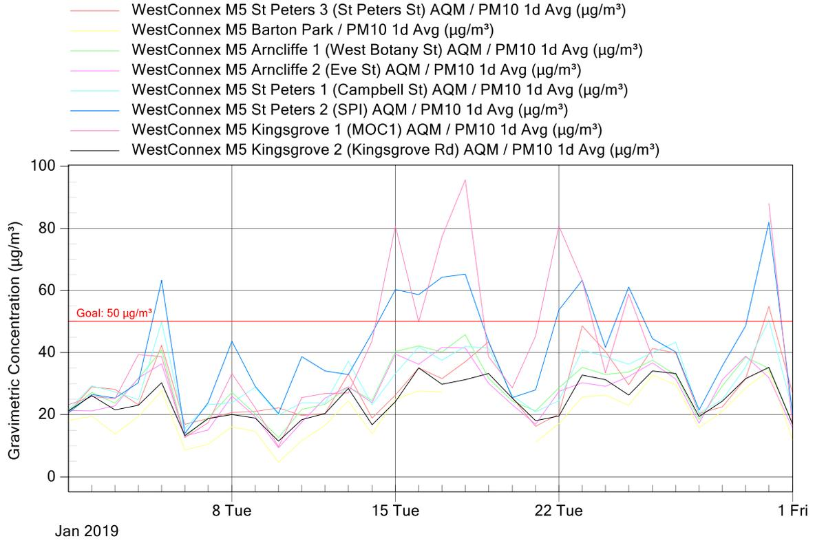
Figure 4: New M5 Project Air Monitoring Stations - PM<sub>10</sub> 24 Hour graph for January 2019
