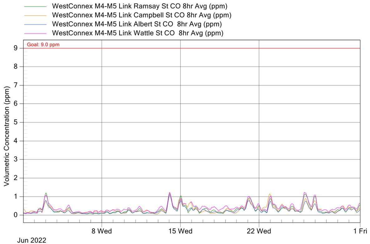
**Figure 2: WCX M4-M5 Link Project Air Monitoring Stations - CO 8-Hour Rolling Graph for June 2022**
