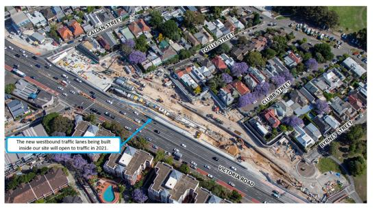
The new traffic lanes and shared path on Victoria road are expected to open in early 2021, before construction moves to the middle lanes on Victoria Road to build the tunnel entry and exit portals.
