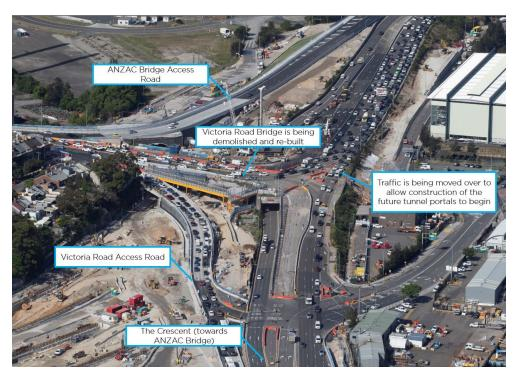
The aerial picture on the left shows the new temporary roads in operation around the Victoria Road/The Crescent intersection. Traffic has been moved onto these temporary roads so we can start to demolish and reconstruct the Victoria Road bridge.
