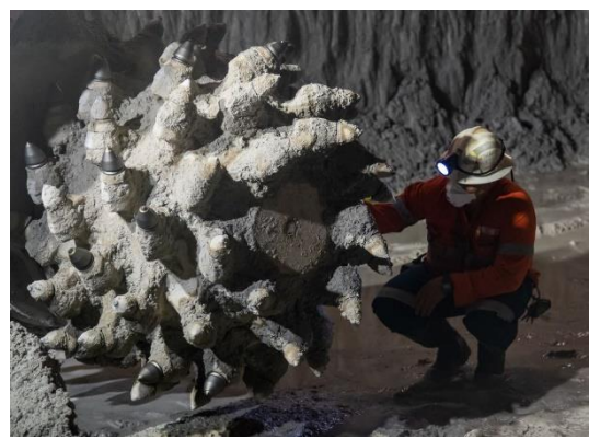
Photo of the cutting end of the roadheader. The 'teeth' gradually cut into the rock in a circular motion and as a result, need to be frequently replaced!
