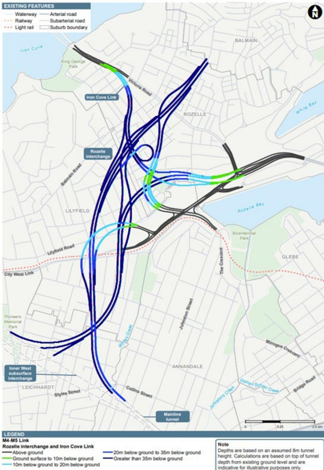
Figure 6-12 Indicative tunnel depths - Rozelle interchange and Iron Cove Link
