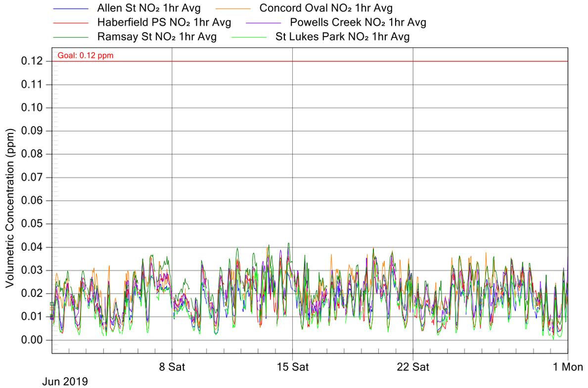
Figure 3: M4 East Project Air Monitoring Stations - NO<sub>2</sub> graph for June 2019
