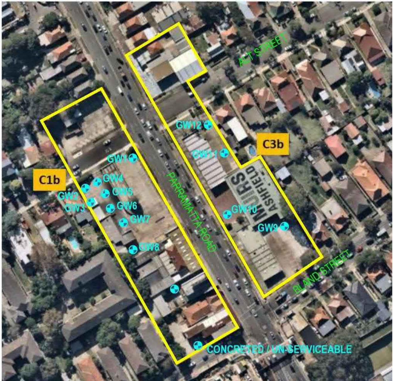
The Epic 2018 PSI conducted a groundwater monitoring event (**GME**) on 9/08/18 that involved measuring the standing water level (**SWL**), total depth and screened interval for each pre-existing well. Three additional groundwater monitoring wells were installed by Epic as part of the DSI and a second round of well dipping was conducted on 20 - 21/11/2018. A summary of groundwater monitoring data obtained by the PSI for the pre-existing and new wells is presented in **Tables 2-12 and 2-13**.
