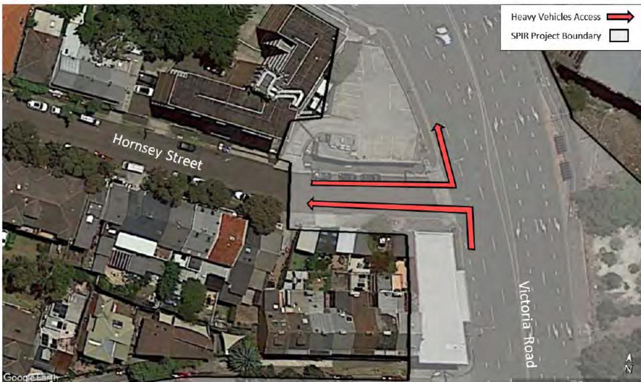
Note: Heavy vehicle access to/from Victoria Road (red arrows) will occur when Hornsey Street is open to the public, in accordance with an approved Traffic Management Plan with authorised traffic controller(s).
