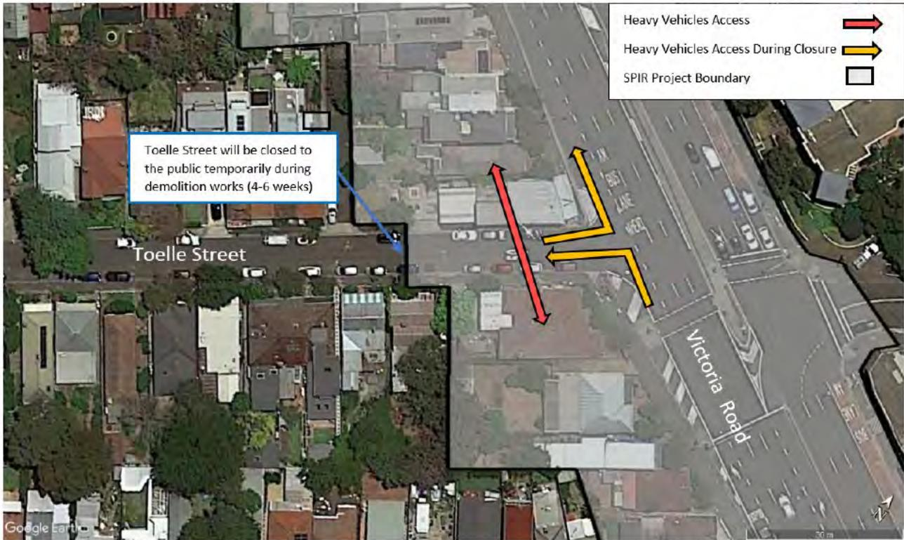
Note: Heavy vehicle access to/from Victoria Road (yellow arrows) will occur within the Project boundary, when Toelle Street is closed. Heavy vehicle crossing of Toelle Street (red arrow) will occur when Toelle Street is open to the public in accordance with an approved Traffic Management Plan with authorised traffic controller(s).
