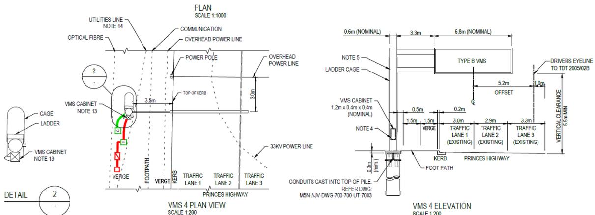
Figure 3. VMS4 plan and elevation view with surrounding services
