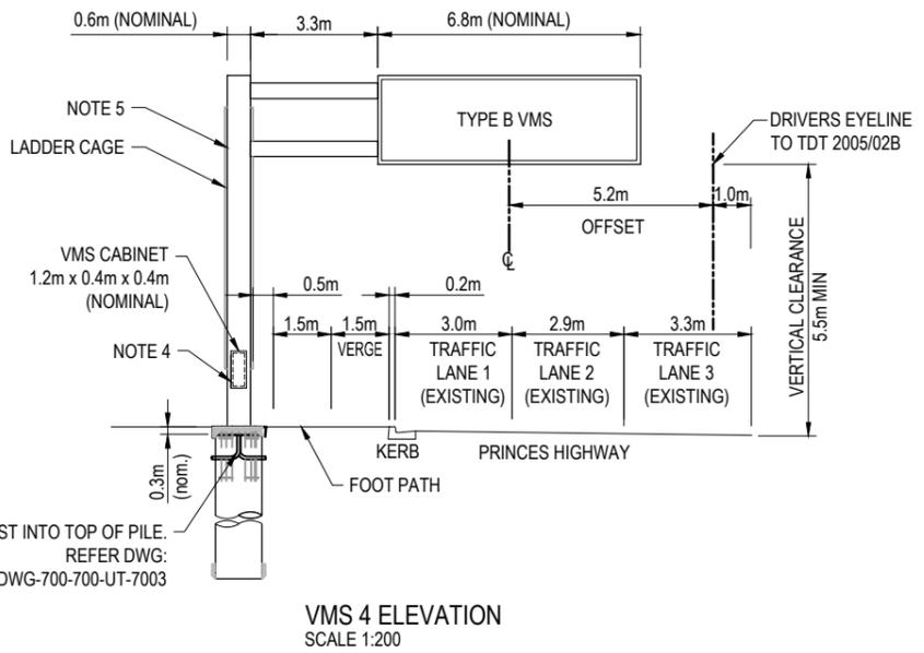
CONDUITS CAST INTO TOP OF PILE.
