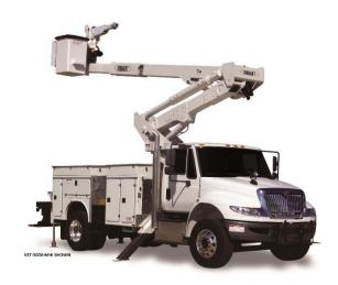
**Image:** a bucket truck used by technicians for overhead powerline work.
