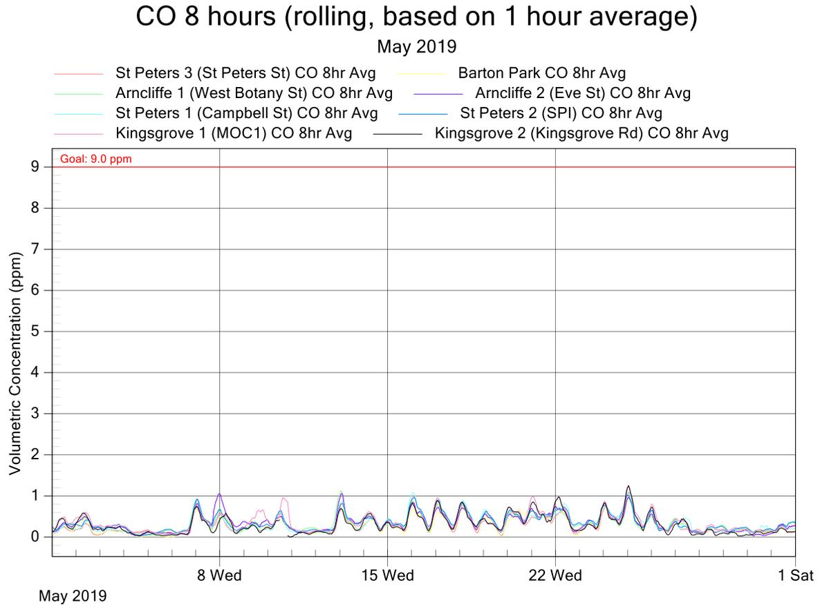
Figure 2: New M5 Project Air Monitoring Stations - CO 8 hours rolling graph for May 2019
