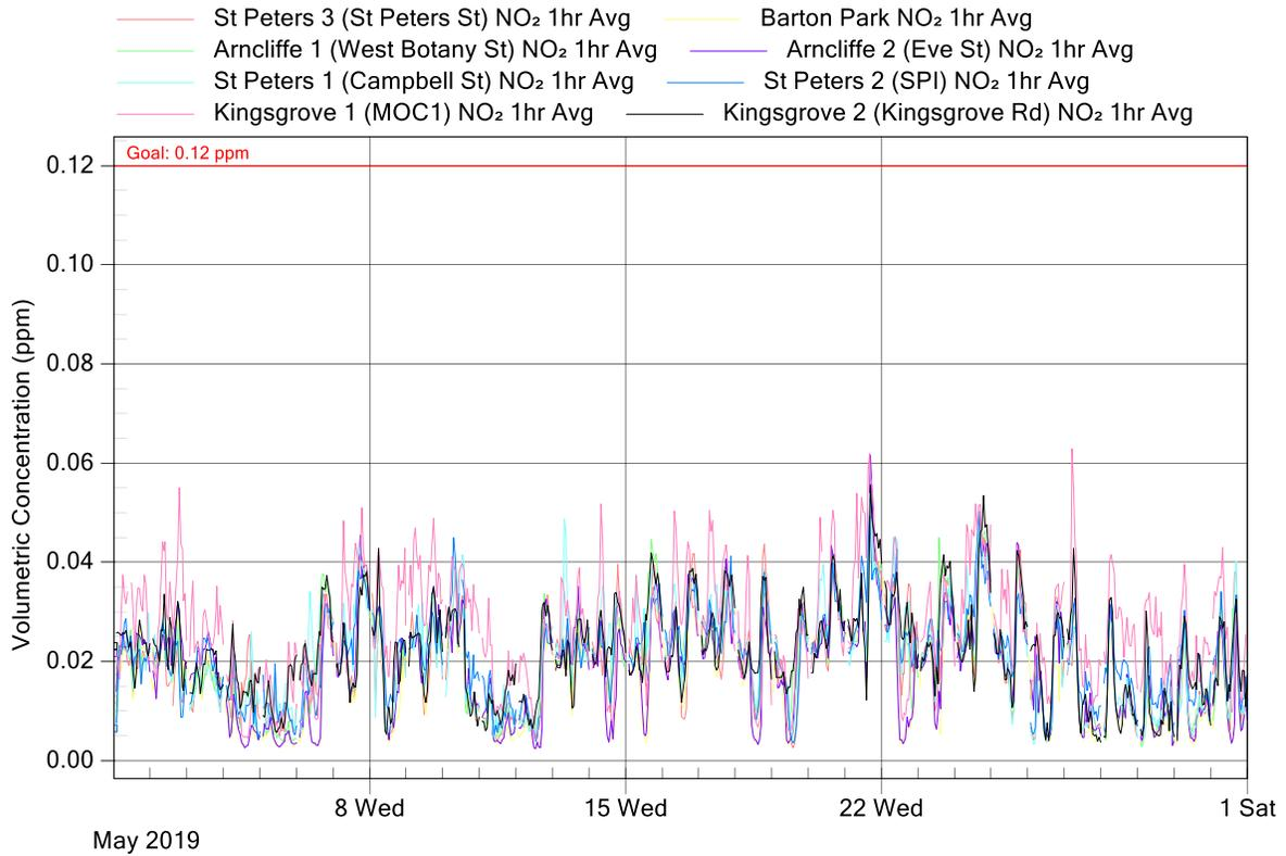
Figure 3: New M5 Project Air Monitoring Stations - NO<sub>2</sub> graph for May 2019
