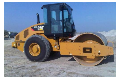
Vibratory rollers are used to compact and smooth new asphalt
