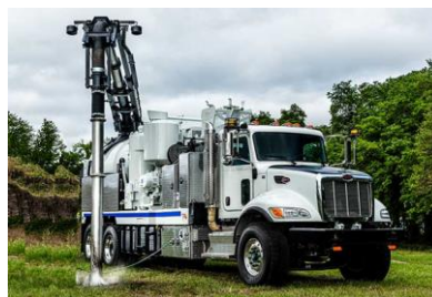
Vacuum trucks are used to suck up soil, small stones and water around the area of work
