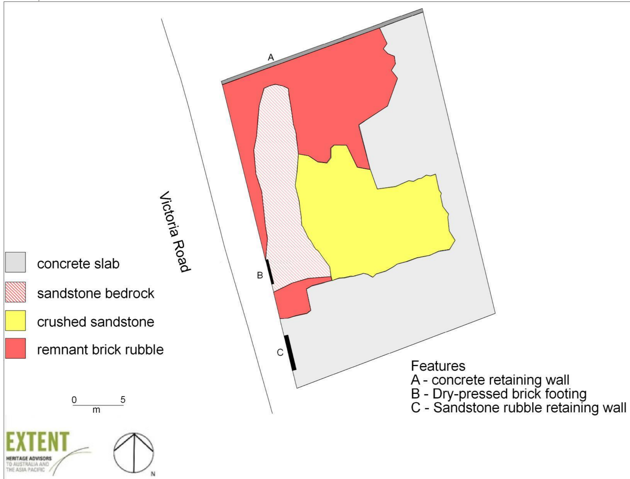
Figure 4 White Bay Hotel site – surface features
