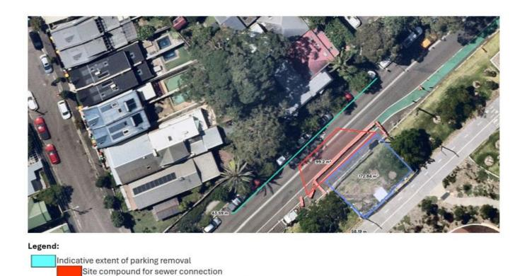
Figure 5-2 Additional scope to facilitate utilities connections of new public toilet block
