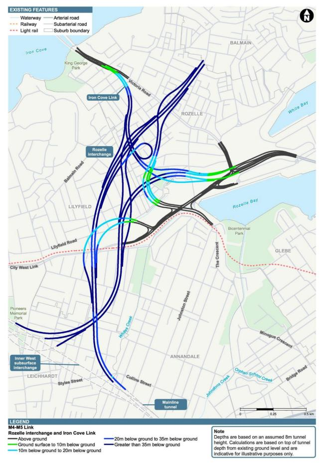
Figure 1-2 Overview of the Rozelle Interchange
