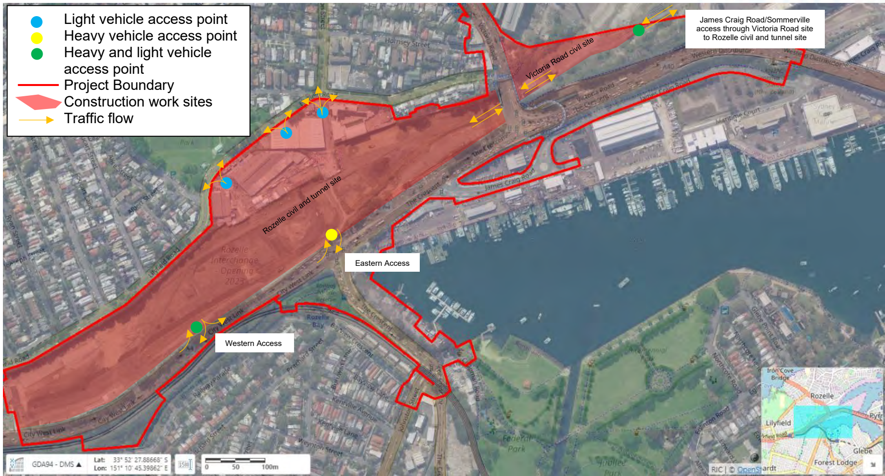
Figure 1 Vehicle access locations at the Rozelle civil and tunnel site (C5)
