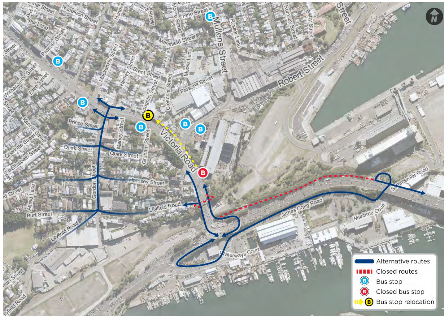
Figure 20 Stage 1 Pedestrian and cyclist routes – Hornsey Street and Victoria Road bridge removal
