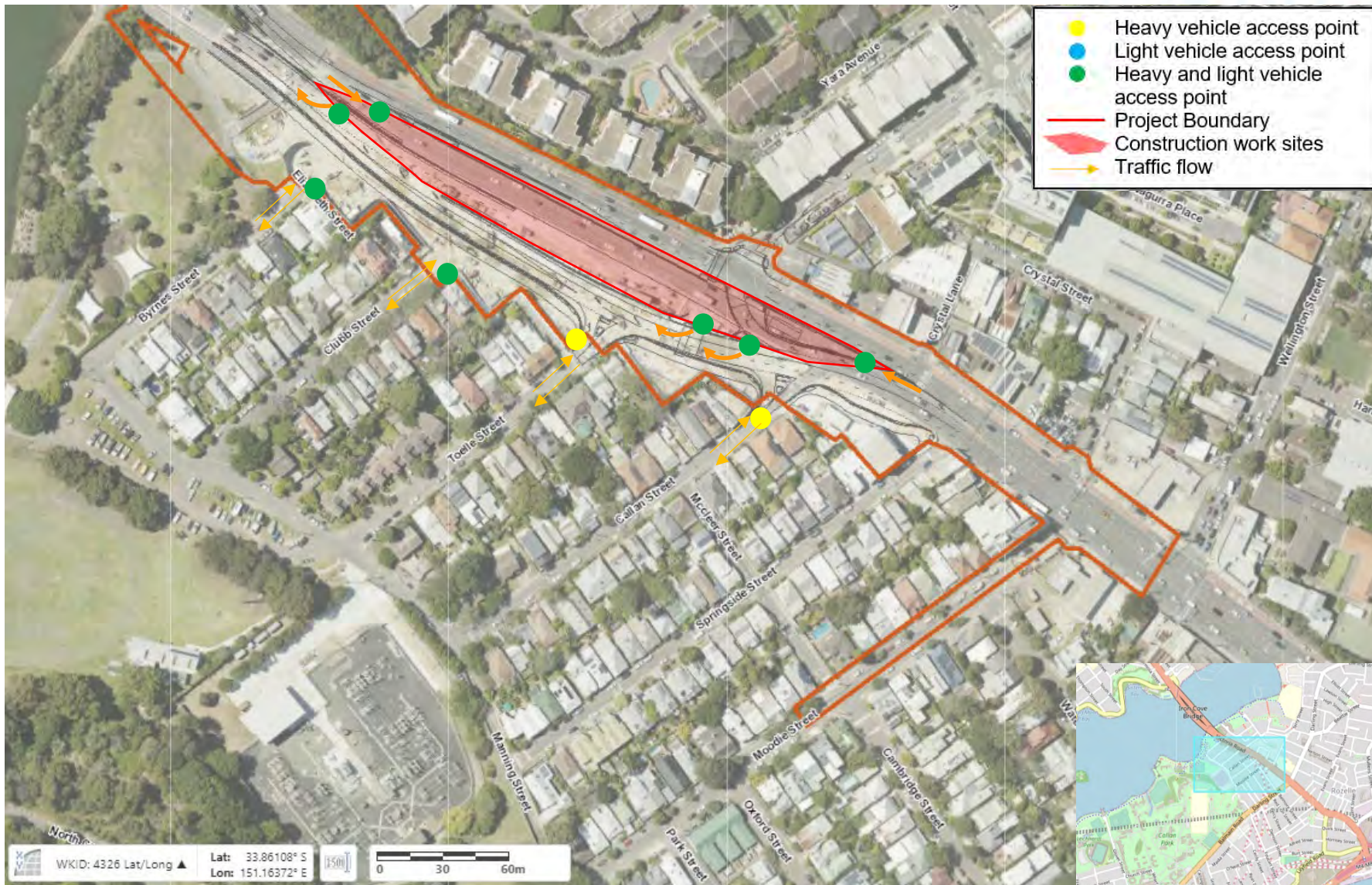
Figure 5 Vehicle access locations at the Iron Cove civil site (C8) - Stage 2
