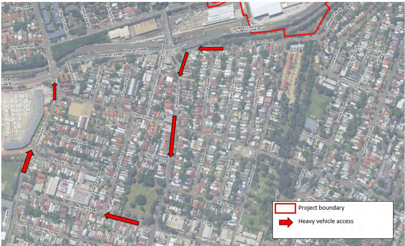
Figure 14 Catherine and Brennan Street – exit. Note the route proceeding down Catherine and along Moore Street is subject to a differing heavy vehicle maximum limit being 22 heavy vehicles per day, maximum 6 heavy vehicles per hour.
