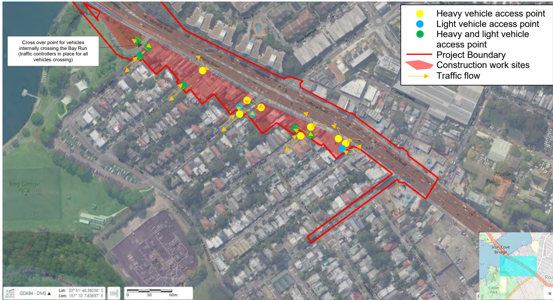
Figure 4 Vehicle access locations at the Iron Cove Link civil site (C8)
