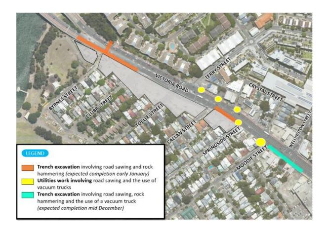
**Equipment used:** for night work includes but isn't limited to: road saws, vacuum trucks, excavators with hammer attachments, compaction machines, hand tools and construction vehicles.
