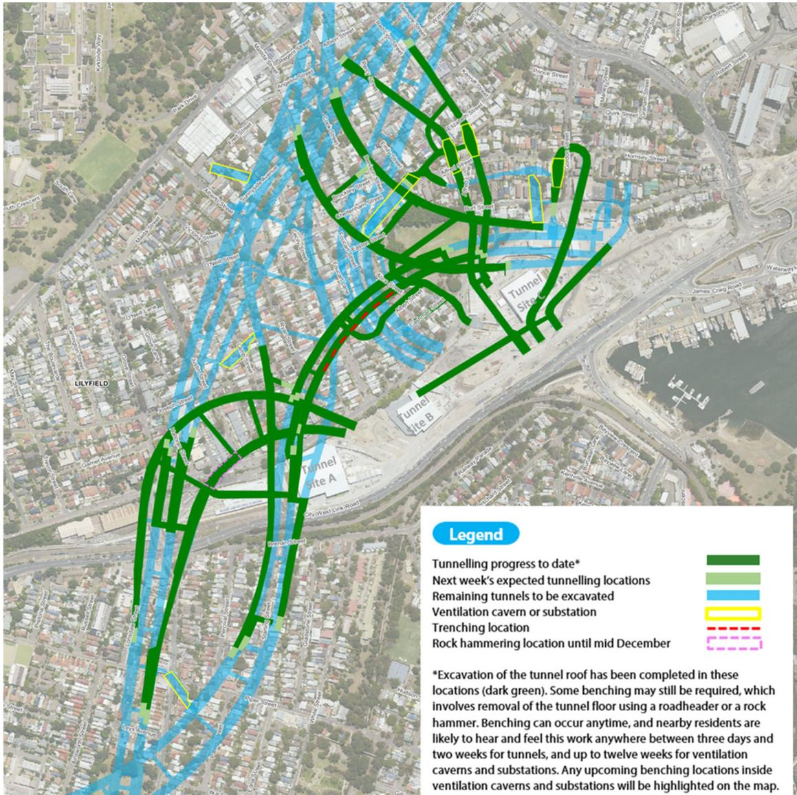
In recent weeks we've started digging stormwater drainage trenches inside some of the already excavated tunnels; upcoming trenching locations are shown with a **red dashed line** on the map above.
