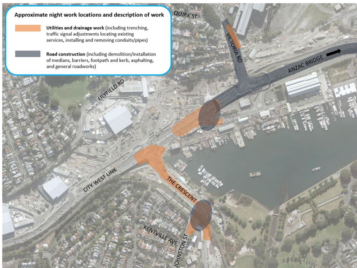
The above night time activities will involve the intermittent use of road saws, rock hammers, asphaltting machines, rattle guns and linemarking removal equipment. These activities are expected to
