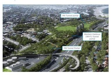
As you may have already noticed, the construction site is currently lower than Lilyfield Road allowing us to build the portals from the ground up. Once we've completed construction of these portals and associated structures within the Parklands, we'll start backfilling the whole area so that it becomes level in most places, with Lilyfield Road.
