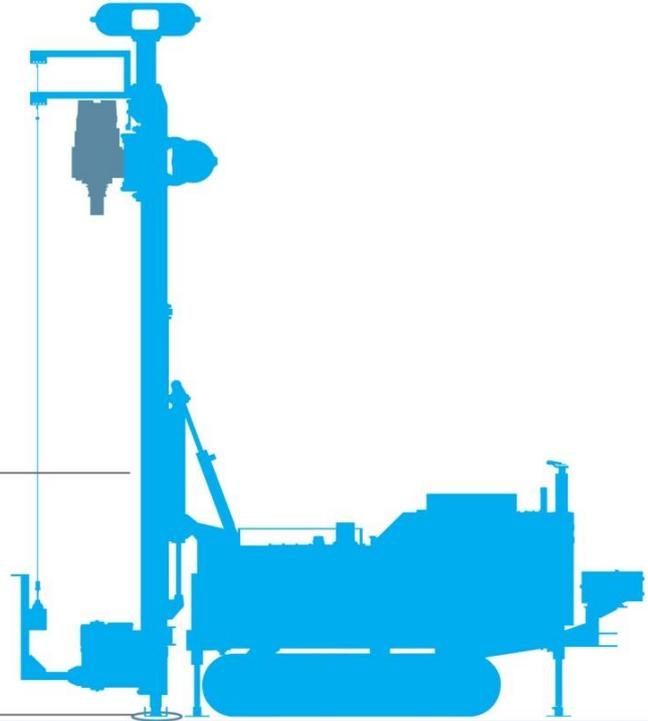
**Drilling rig** used to collect samples to produce a geological profile of the area. The rig size may vary depending on the ground condition and the drilling depth size.
