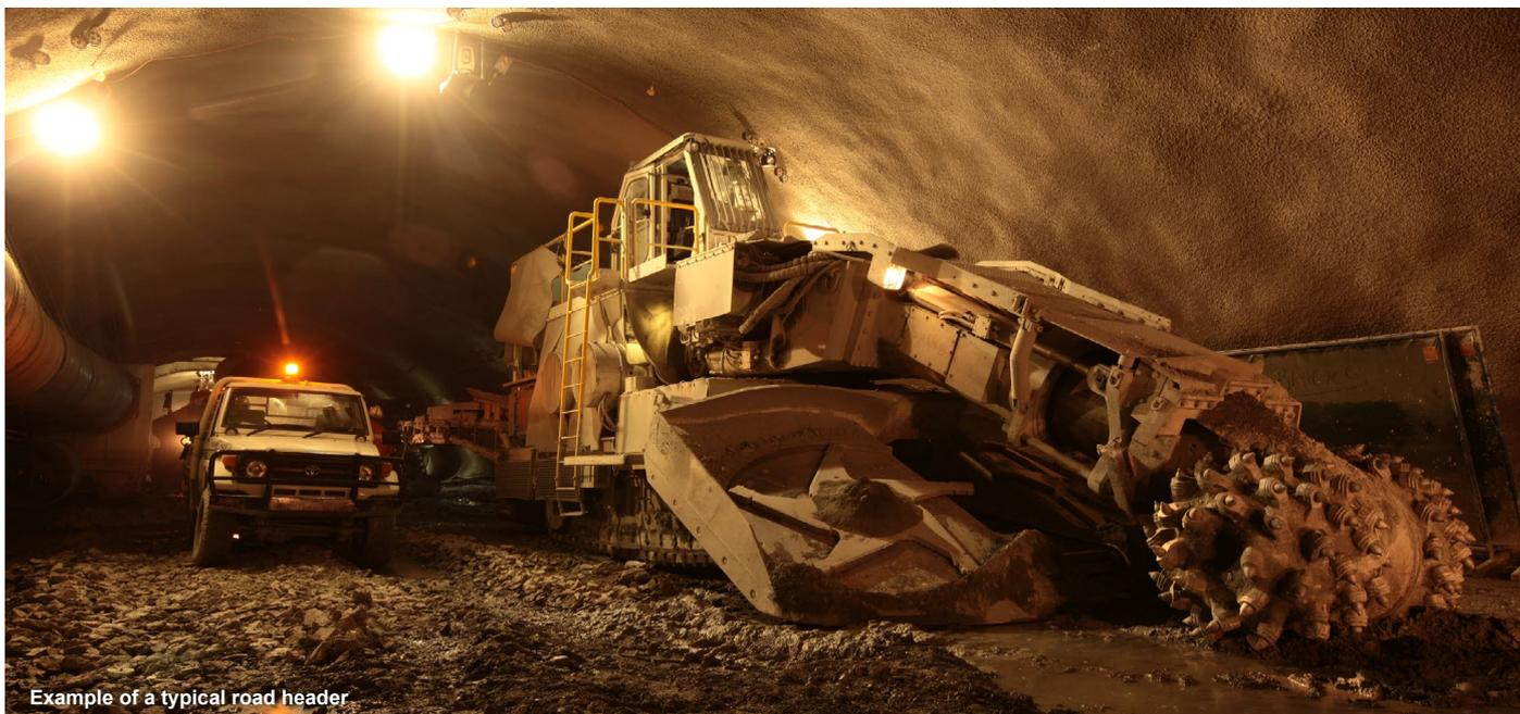
Example of a typical road header
