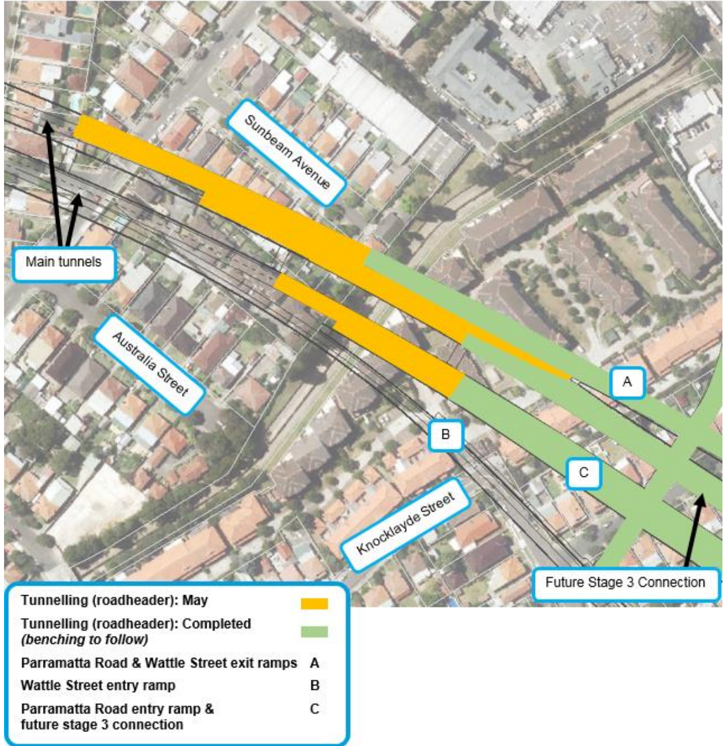
Location of tunnelling activity – Northcote Street construction site.
