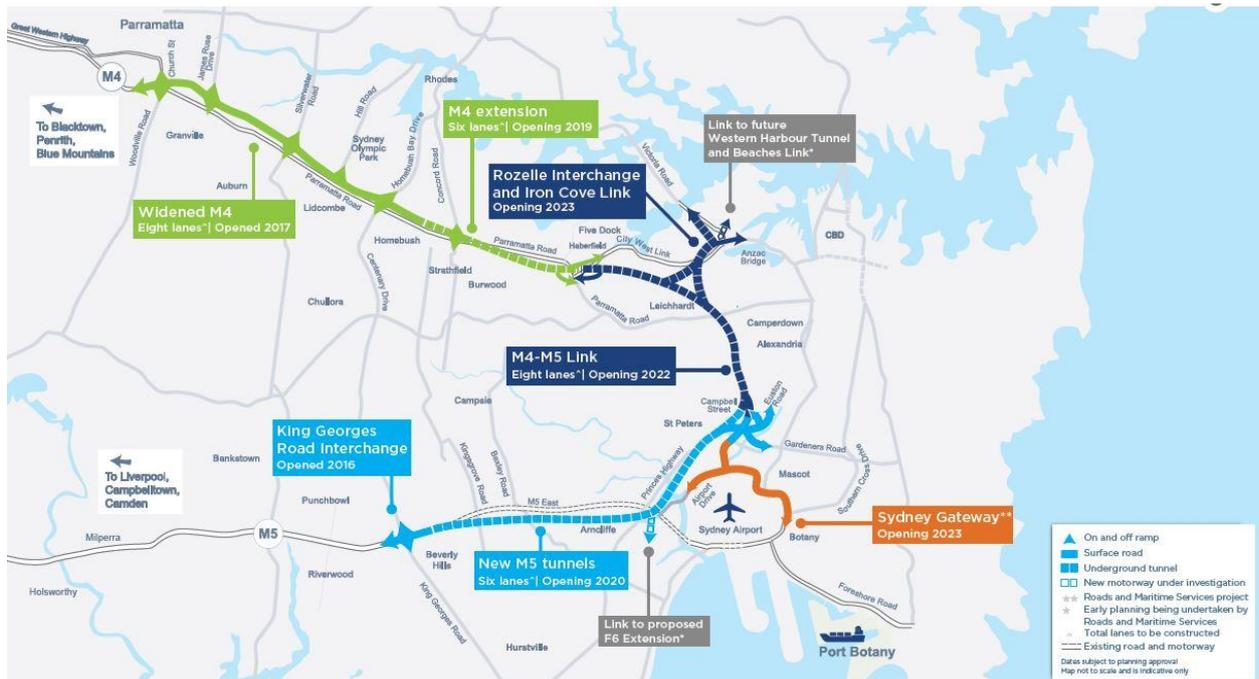
The New M5 Project (New M5, the project) is designated as State Significant Infrastructure (SSI 6788) and is the Stage 2 component of the WestConnex scheme. The proponent for the project is Roads and Maritime Services (RMS) and the project company (WCX M5 AT). WCX M5 AT has engaged the CPB Samsung Dragados Joint Venture (CDS-JV) to deliver the design and construction of the project. The project was approved by the Minister for Planning on 20 April 2016, subject to conditions.
