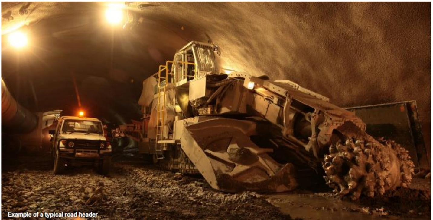
Example of a typical road header
