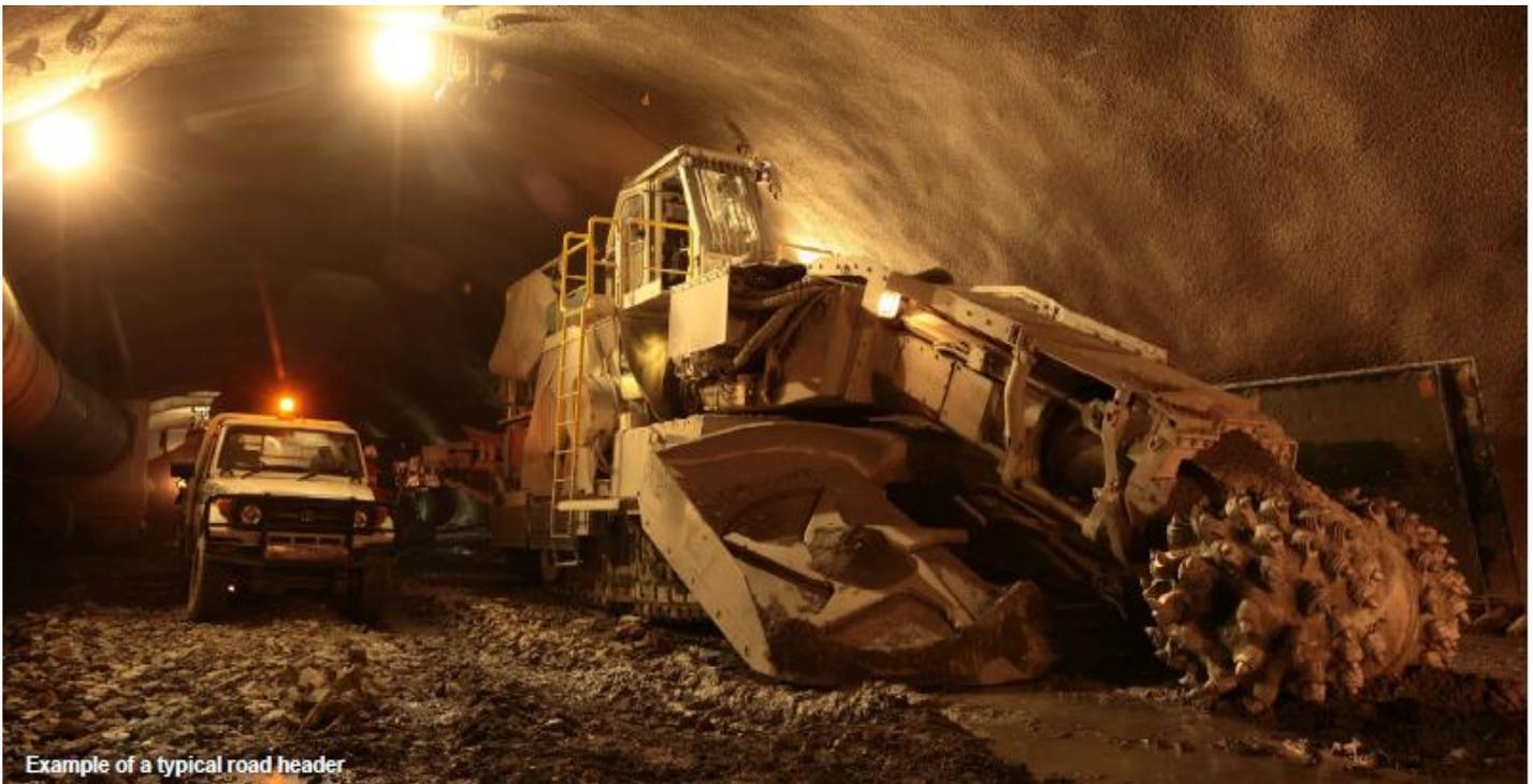
Example of a typical road header
