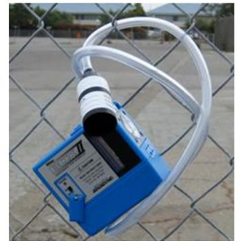
An asbestos monitor fixed to a fence at the St Peters Interchange site
