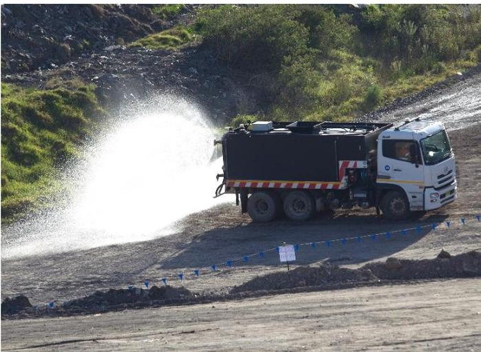
Water carts are used to spray recycled water onto haul roads and excavation areas
